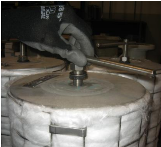
Push the threaded down and turn the lever counterclockwise to release the Fiberwind™ elements
