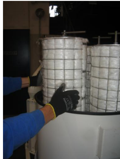
Lift the filter elements (12kg/ea) manually or using a hoist and extract them from the vessel.
