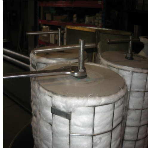
Loose the fixing nut completely.
