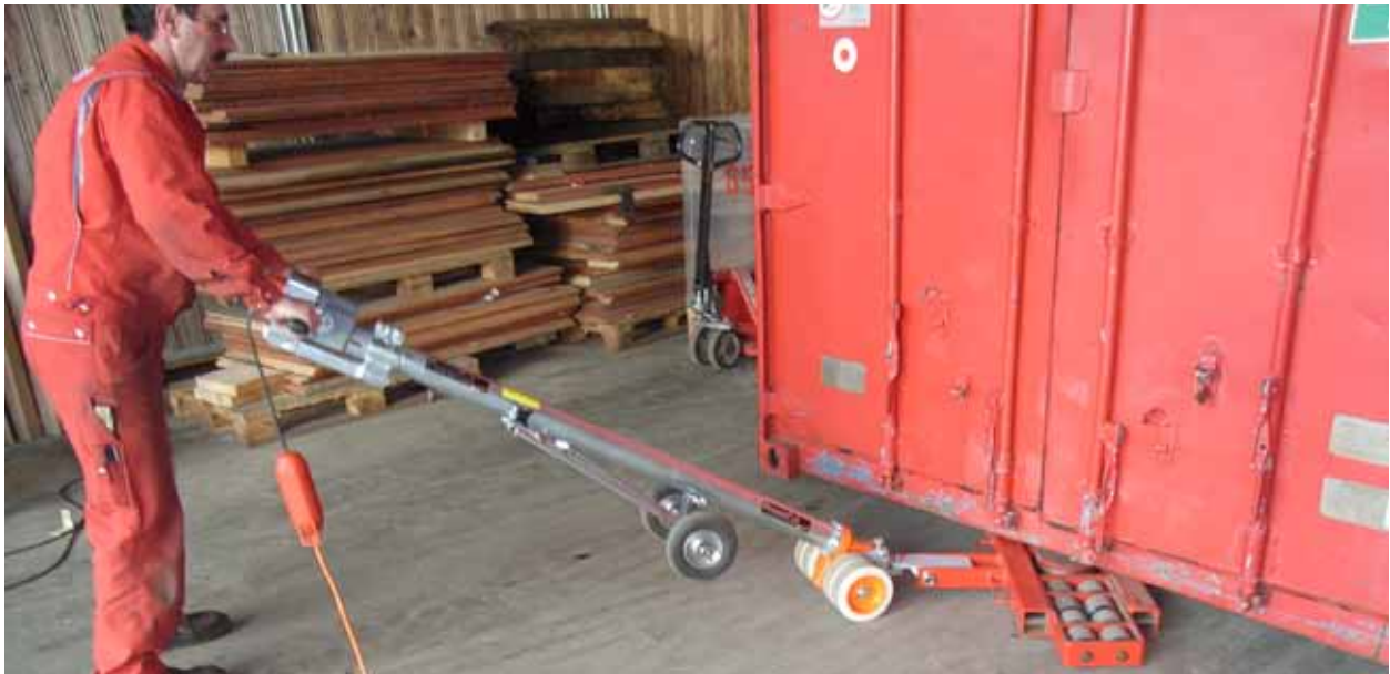
Job example: PowerAttack hooked up to a steerable skate with folded aux-trolley moving a container!
